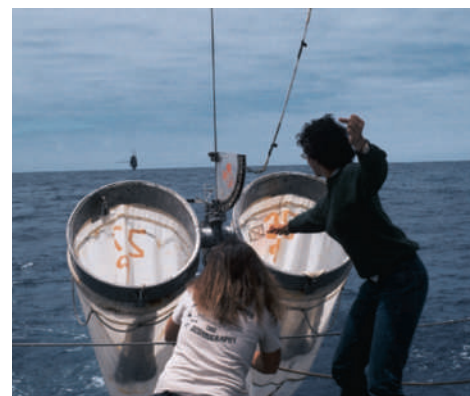
FIGURE 1.3 These marine scientists are hauling in a net known as a “bongo net” used to capture minute marine plankton. One is signaling instructions to the winch operator.
